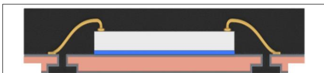
Fig. 2. Step cut wirebond MLF ® cross sectional view. Wires extend from the die pads to the leadframe with loop geometry.
