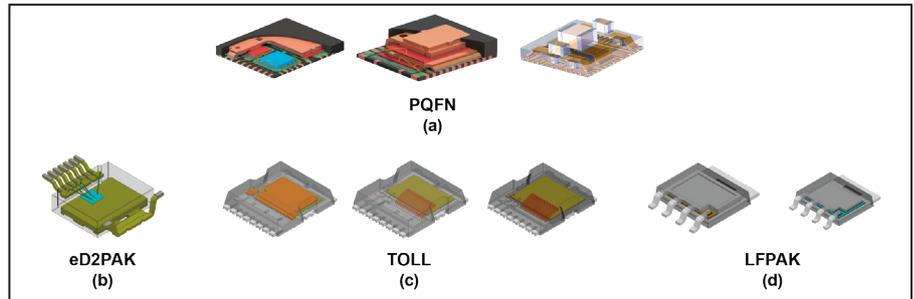
**Figure 1:** Available power discrete capabilities include: a) PQFN evolution, b) eD2PAK with heat spreader tab, c) TOLL variations, and d) LFPAK.
