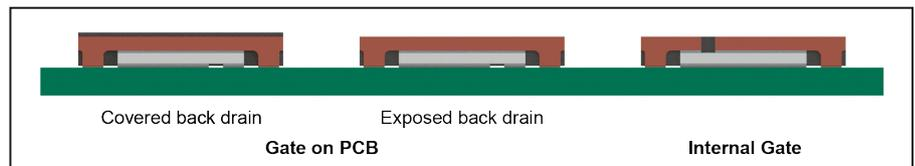
**Figure 4:** The PowerCSP™ design provides many connectivity options for chip-scale power.
