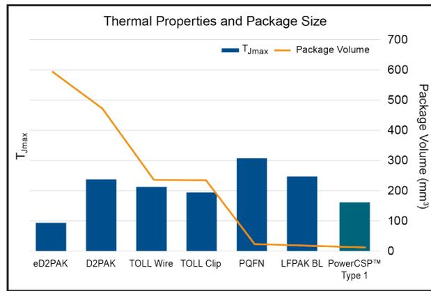
**Figure 6:** Relative junction temperature vs. package volume for various power packages.
