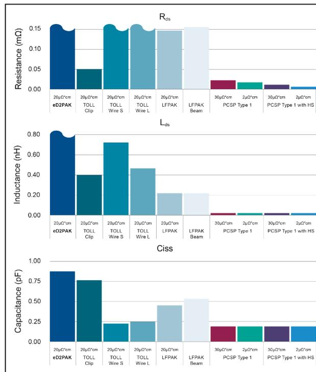
**Figure 7:** Simulated comparison of  $R_{DS}$ ,  $L_{DS}$  and  $C_{iss}$  for the PowerCSP™ (PCSP) design to different versions of eD2PAK, TOLL and LFPK packages.
