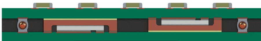
**Figure 9:** Increased integration of power using the PowerCSP™ methodology.
