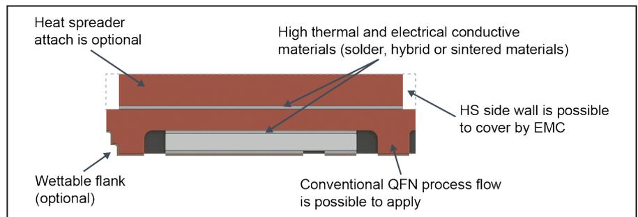
**Figure 3:** The first implementation of PowerCSP™ technology shows its flexibility and many construction options.
