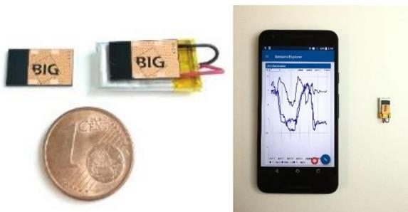
**Figure 10.** SiP soldered directly to Li-Ion Battery (left picture) and smartphone reading SiP sensor data via BLE (right picture).
