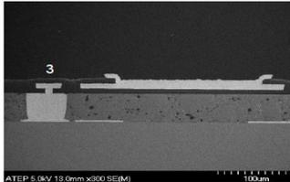
Option 3: Chip last – RDL processed on carrier and chip is assembled on the RDL.
