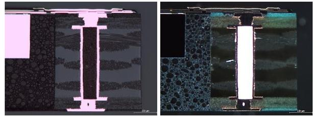
**Figure 8:** Shared TPV – package’s left side (left: brightfield; right: darkfield).
