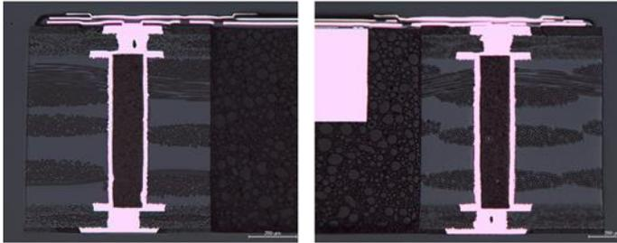
**Figure 14.** Mold compound adhesion to the PCB vias.
