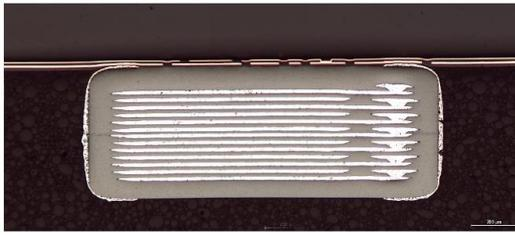
**Figure 13.** Mold compound adhesion to the surface mount devices (SMDs).
