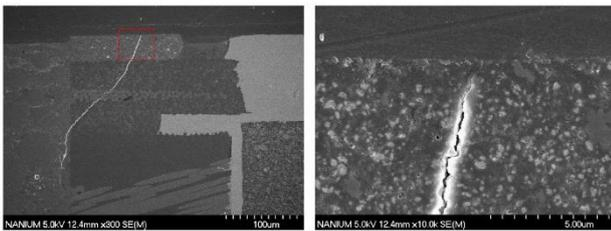
**Figure 15.** Cracking in the PCB via and interface PCB to mold compound.
