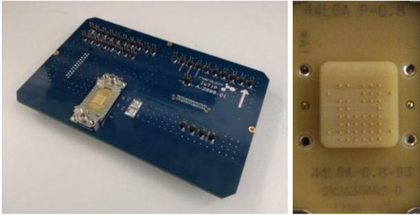
**Figure 9.** SiP test load-board and socket.
