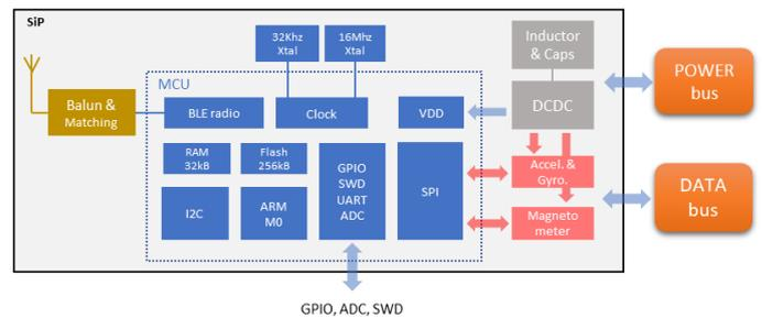
**Figure 2.** SiP block diagram.
