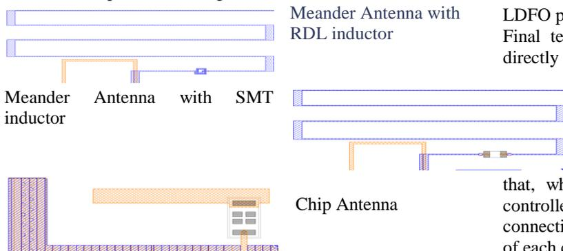
**Figure 7:** Antenna types in the test vehicle.
