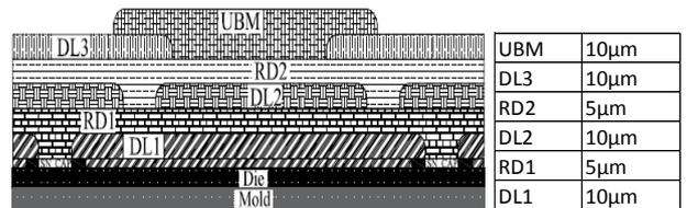
Typical RDL stack-up for the backside RDL is:
