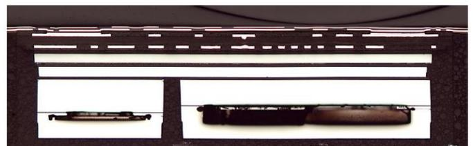
**Figure 12.** Cross sections of mold to mold interface of pre-molded packages.
