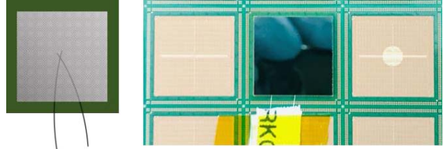
Figure 3. Thermocouple kit: the thermocouple wire is located in the center of the die bump area.
