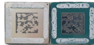
Figure 14. Lid pull test of graphite sheet TIM after reliability test.
