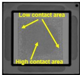
Figure 9. CSAM image of graphite sheet TIM post reliability test (HTS 1000 hrs). Dark black indicates high contact on lid. White spots indicate low contact on lid. 90% TIM coverage with 10% voids.
