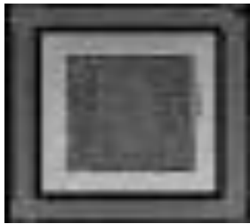
Figure 8. CSAM image of In10Ag-TIM post reliability test (HTS 1000 hrs). White spots indicate voids and dark black indicates overflow. 100% TIM coverage with no voids.
