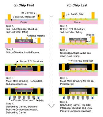
Figure 2. Illustration of Process Flow: a) Chip First; b) Chip Last.
