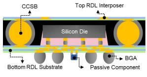
Figure 3. Illustration of RDL-based Interposer PoP with CCSBs
