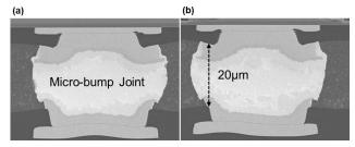
Figure 12. Cross-sectional images of Silicon die mirco-bump joint: a) TC 'B' 1000 cycles with Precon L3 and b) after HTS 1000 hrs.
