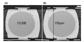
Figure 13. Cross-sectional images of CCSB joint: a) TC 'B' 1000 cycles with Precon L3 and b) after HTS 1000 hrs.
