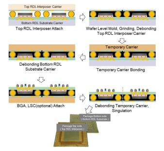
Figure 7. Process flow for RDL-based Interposer PoP with CCSBs.
