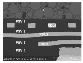
Figure 8. Cross-sectional images of the bottom RDL substrate.
