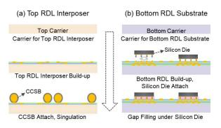
Figure 6. Preparation of (a) top RDL interposer and (b) bottom RDL substrate.
