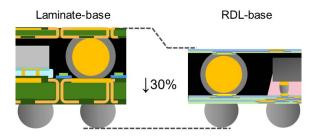
Figure 9. Comparison between a laminated and an RDL-based Interposer PoP
