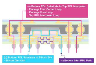
Figure 5. Schematic figure of the three daisy chains' paths.
