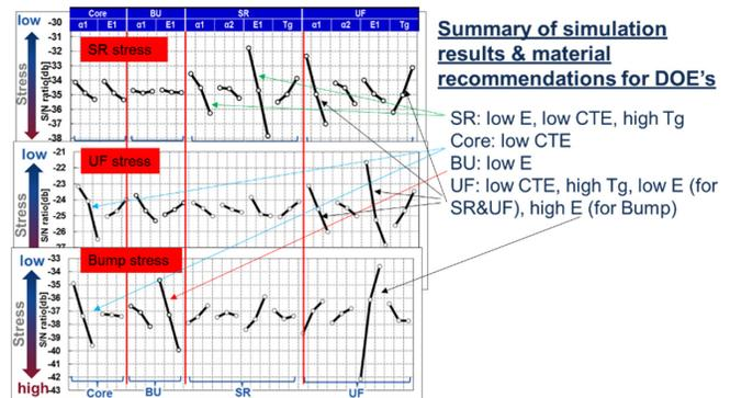
Figure 5. Comparison of impact of material properties on all three mechanisms (SR cracking, UF cracking and bump cracking).
