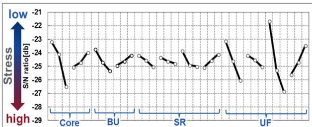
Figure 3. Impact of material properties on UF cracking.
