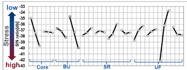
Figure 4. Impact of material properties on chip-interconnect bump cracking.
