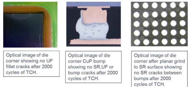
Figure 7. Optical images of units after 2000 cycles TCH showing no evidence of SR, UF or bump cracking.
