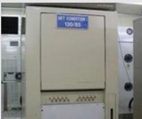
Pressure Cooker Test (Autoclave)
