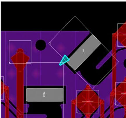
Figure 5: Example of a design rule check violation for component spacing.
