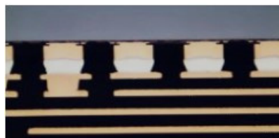
FCBGA chip to chip bonding with Cu pillar
