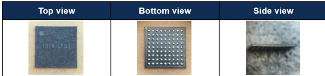
Figure 4) X2FBGA picture after finishing assembly
